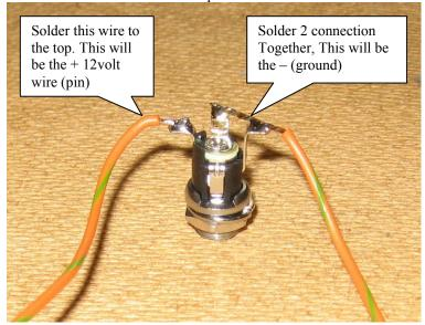
Connect wire to pcb, watch out you mount the + and – the good way (Wrong way connection is protected by D1, if it does not work connect the 2 wires around)
