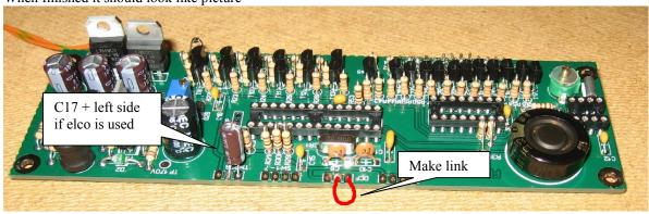
Thrue small designer mistake you have to make a modification with two wire connections on the pcb. The cutting of pcb lines is already done. The thin blue wire is included in kit.
