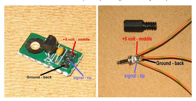
Make 3 wires of 15cm, or use own cable to make any length. You also can decide to use no wire and mount pcb straight on the 3.5mm plug. (you can buy 3.5mm jack-jack cable of any length, cut of one plug and connect pcb.)
