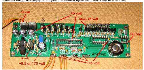
Measure the voltage on +V this should be around 12Volts dc
